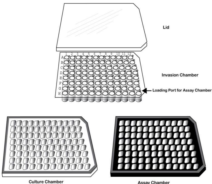
**Figure 4. Diagram of Trevigen's 96 Well version of the High BME Cell Invasion Chamber and assay plates.**
